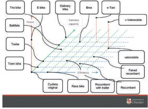
Over time, it seems that the bicycle, originally meant to go from point A to point B in a cheap way, has developed to meet various needs, such as delivery of goods (capacity), speed (efficiency) and comfort (power), as seen in the figures above. One can see that *the latest ideas and developments, such as the e-taxi and the e-velomobile, are aiming at meeting those three human needs: moving people and goods in an comfortable and efficient manner.*
